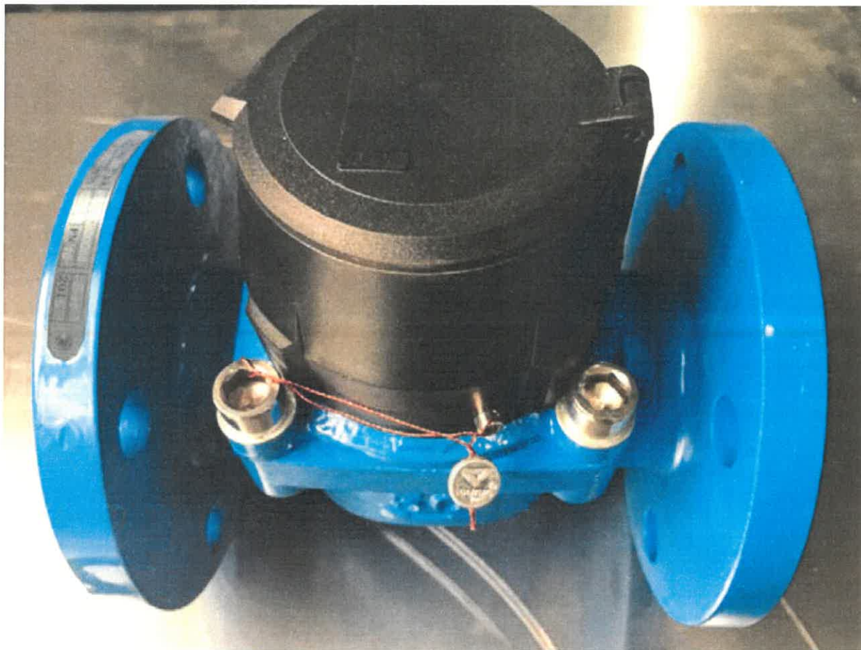
Figure 1: The water meter type LXLC – view and sealing:
